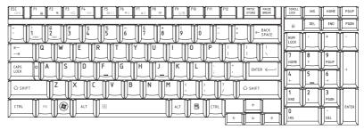
Figure 5-1 A 104-key enhanced keyboard layout
